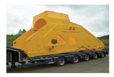
Main ramp of the machine for bending pipes (for the construction of pipelines)
