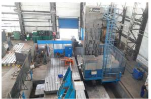
$\begin{array}{c} \text{machining space X x Y x Z x V} \\ 12500 \ x \ 5000 \ x \ 2300 \ x \ 2000 \ \text{mm} \end{array}$
